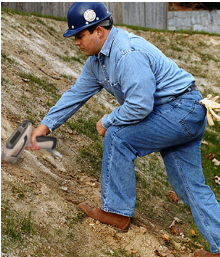
Figure 1-1. In-Situ Soil Testing
