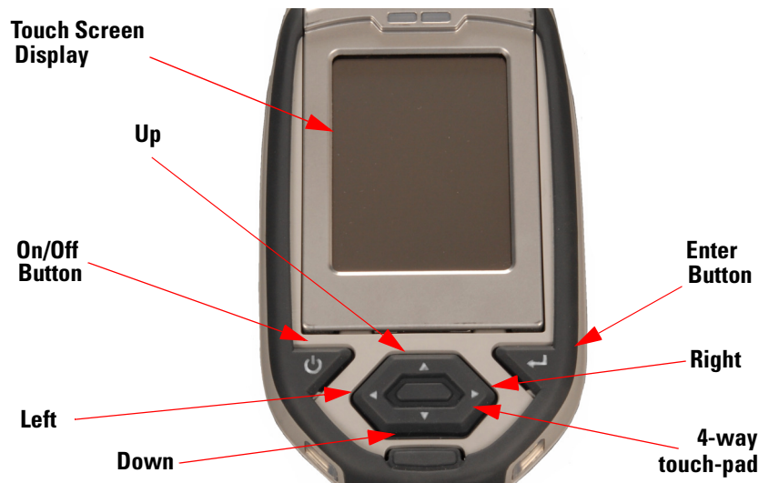
Figure 1-7. The Control Panel
